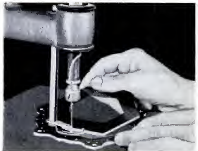
The frame is cut out on a jigsaw, above, using a fine-toothed blade. Below, the frame is set in a vise and strung with wire. To finish the assembled trivet, polish with fine steel wool and coat with lacquer
